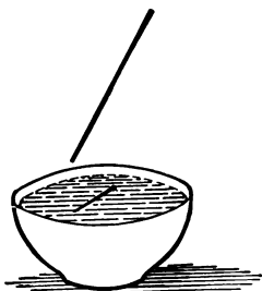
FIG. 92. A magnetized sewing-needle floating on a bowl of water.
